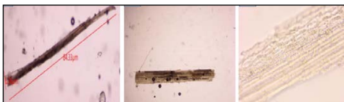
Figure 5: Optical microscopic images of cellulose extracted from sugarcane bagasse, including measurements and images at different magnifications
