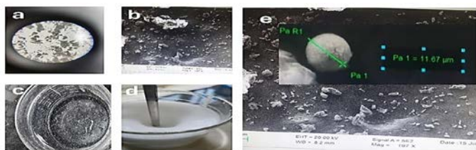
Figure 3: shows the levofloxacin floating microballoons in the following views: (a) microscopic, (b) normal, (c) floating, (d) emulsion development, and (e) SEM picture of the floating microballoons.
