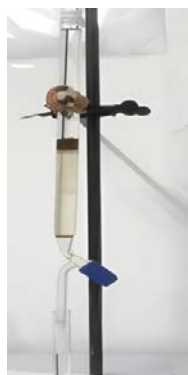
Figure 2: Isolation of components by column chromatography
