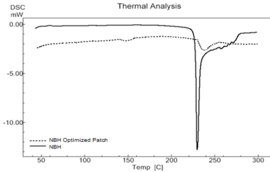
Figure 2: Differential scanning calorimetry of pure drug Nebivolol hydrochloride and transdermal patch
